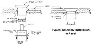
To install CA2025 or CA2035 retaining ring on stud nut, insert pilot of tool completely into stud nut threads and slide the retaining ring onto the stud nut.
